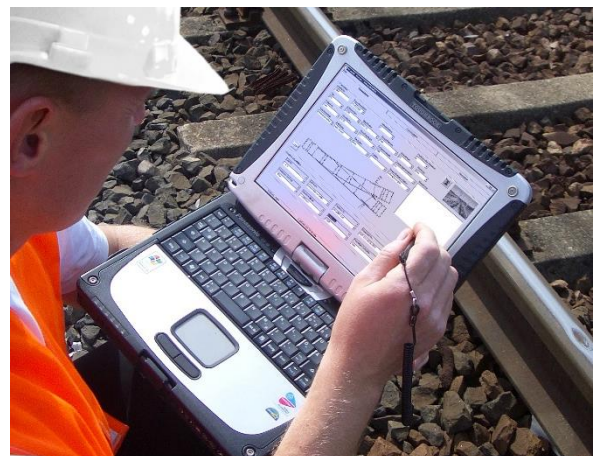
Figure 11: Secondary inspection of track with MR.pro®
