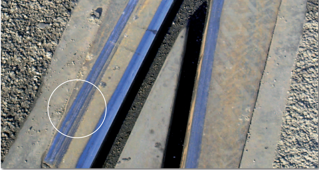
Consequences of inadequate wheelset maintenance. Hollow wheel profiles cause massive beating sounds.
