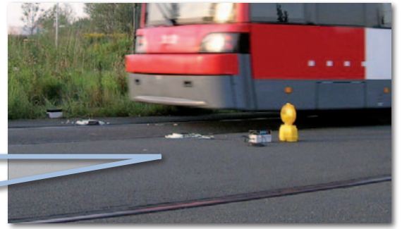
The DigiLot® measurement system developed by Rhomberg Sersa Service detects horizontal deformations of the wheels to enable accurate recording of track geometry.
